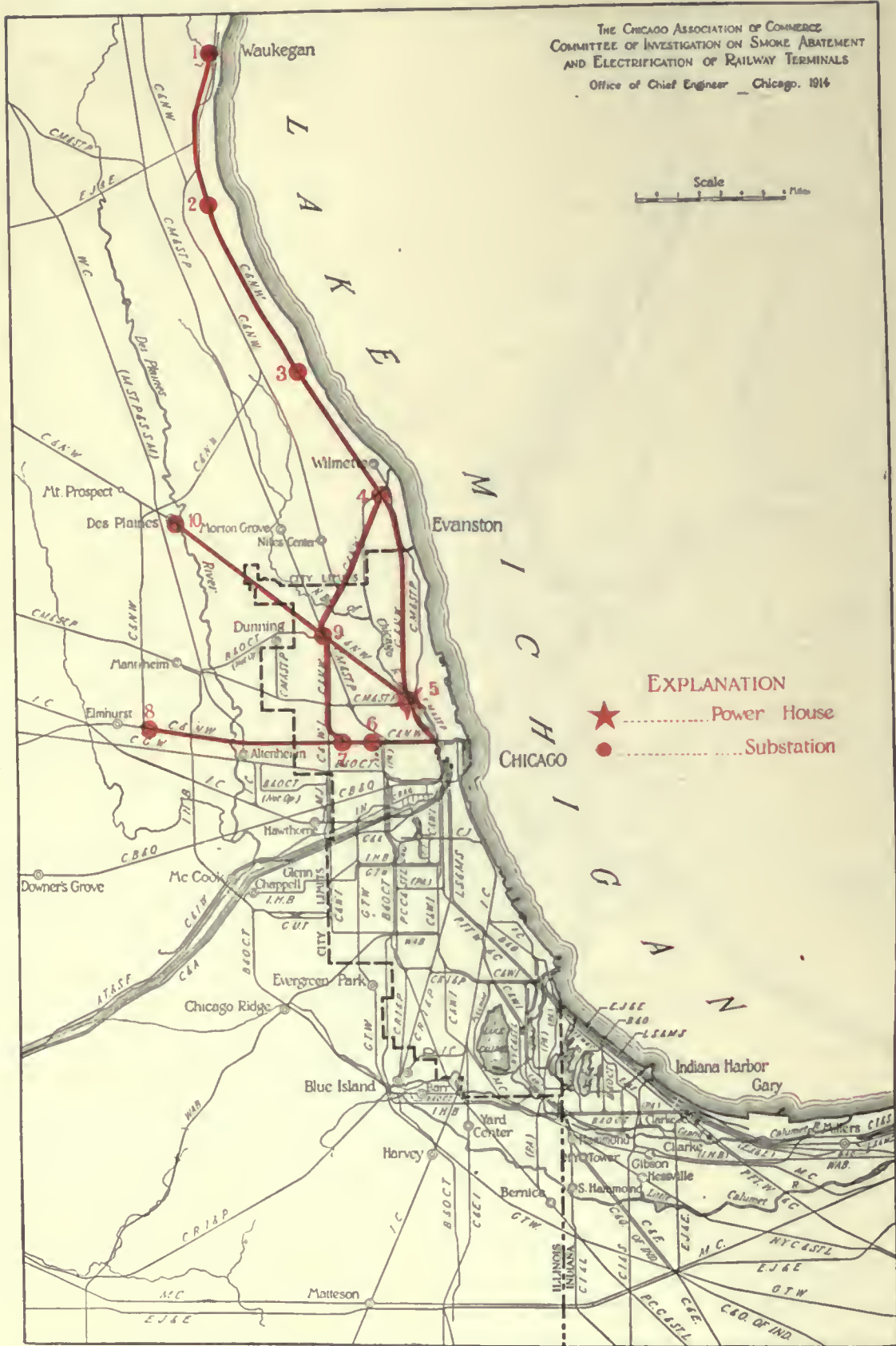
FIG. 686. LOCATIONS OF POWER STATION AND SUBSTATIONS FOR THE 11,000-VOLT A. C. SYSTEM. CHICAGO & NORTH WESTERN RAILWAY
